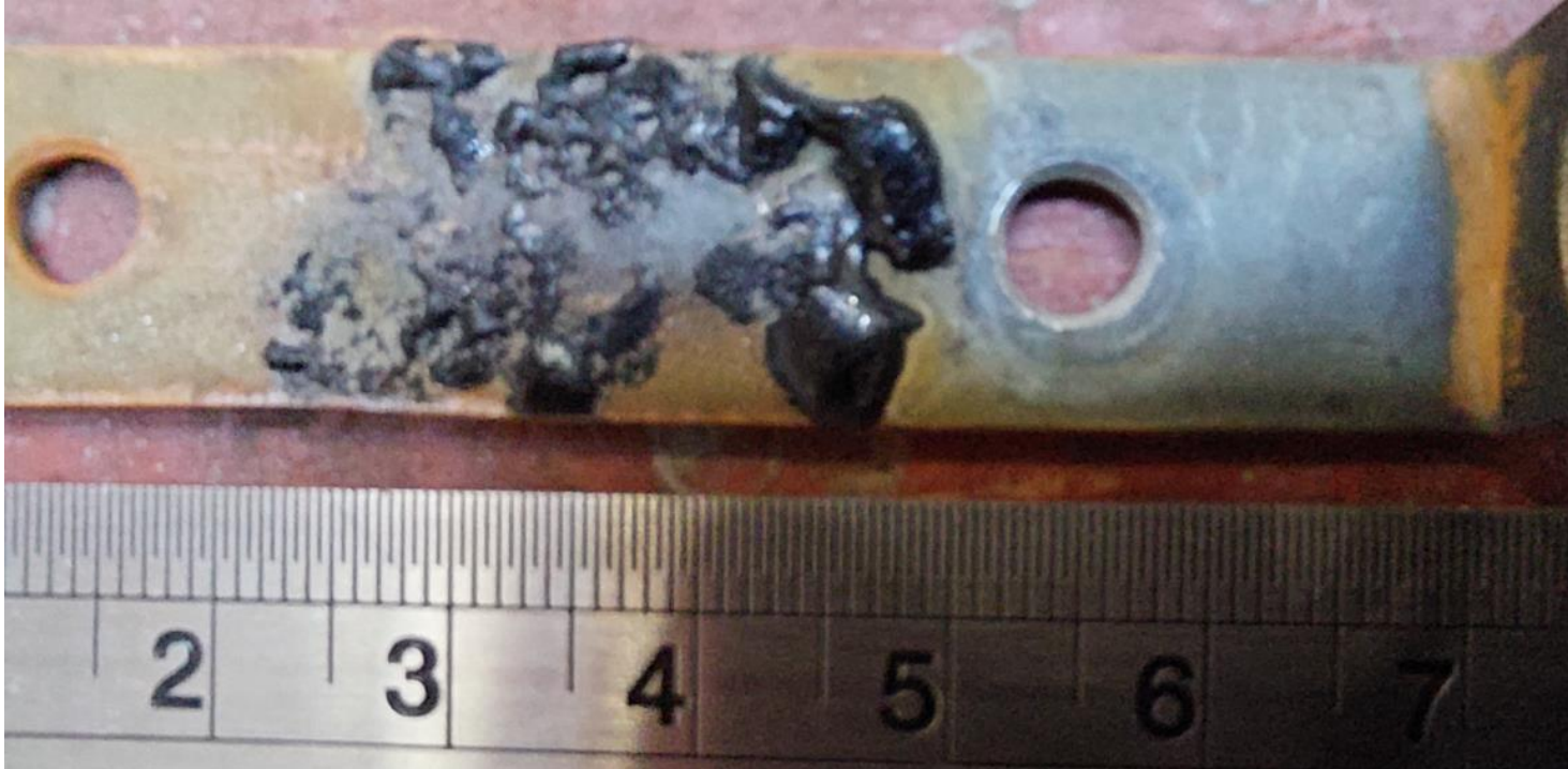
Figure (8): Sample after test with flat (positive) and straight electrodes
