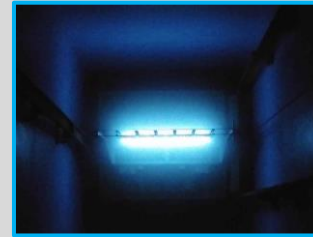
Cherenkov effect around the 25 source rods in the plane rack (activity of around 70 kCi)
